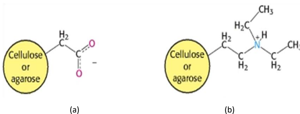
Figure 6. (a) Carboxymethyl (CM) group (ionized form) (b) Diethylaminoethyl (DEAE) group (protonated form)
